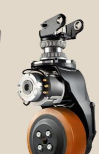
Everything about this drive unit is robust. From the AC motor, to the cast iron gear box with helical gearing, to the tapered roller bearings that secure the drive unit and absorb shock.
