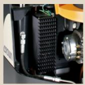
**Sealed high-frequency charger** is designed to operate without a separate cooling fan for even greater reliability.
