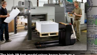
The high-lift fork model raises heavy loads to a comfortable working height to reduce back strain and increase worker productivity.
