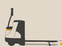
Lift cut-out at full lift protects the motor and pump from continuing to work once full lift is reached. This reduces energy consumption and extends component life.
