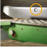
Forks are subject to constant contact with dock boards and irregular surfaces. Crown's pull-rod system places the riser axle at the highest point possible to eliminate damage and wear.
