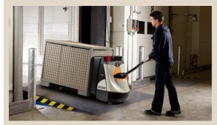
**Crown's ramp hold improves operator confidence and control** by minimising the possibility of unexpected reverse travel when stopped on an incline. It also allows consistent speed on ramps, with or without a load.
